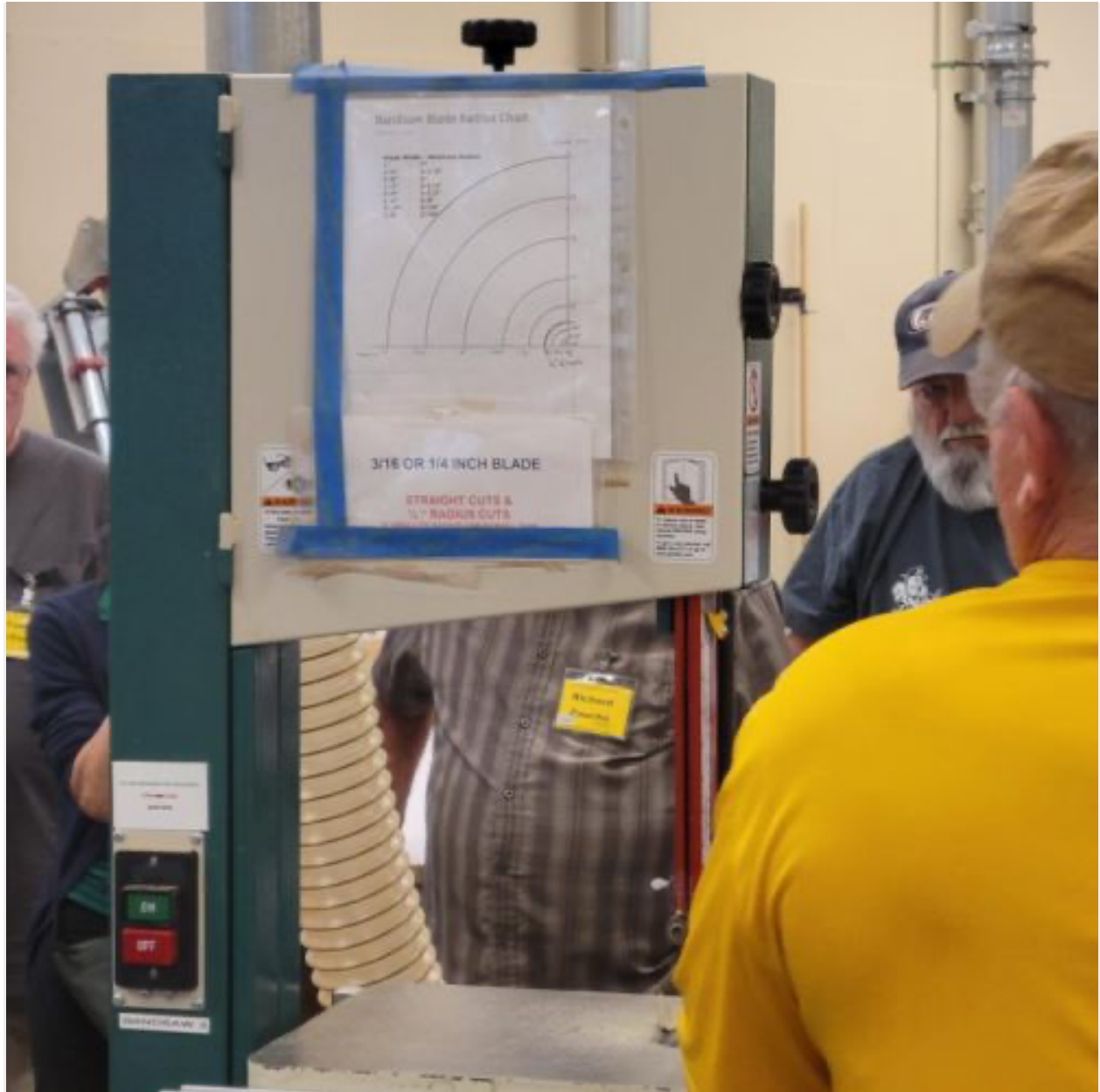
Based on the pencil design, band saw with small blade. The small blade allows for more complete "rounds" "circles" See photo on the band saw.
