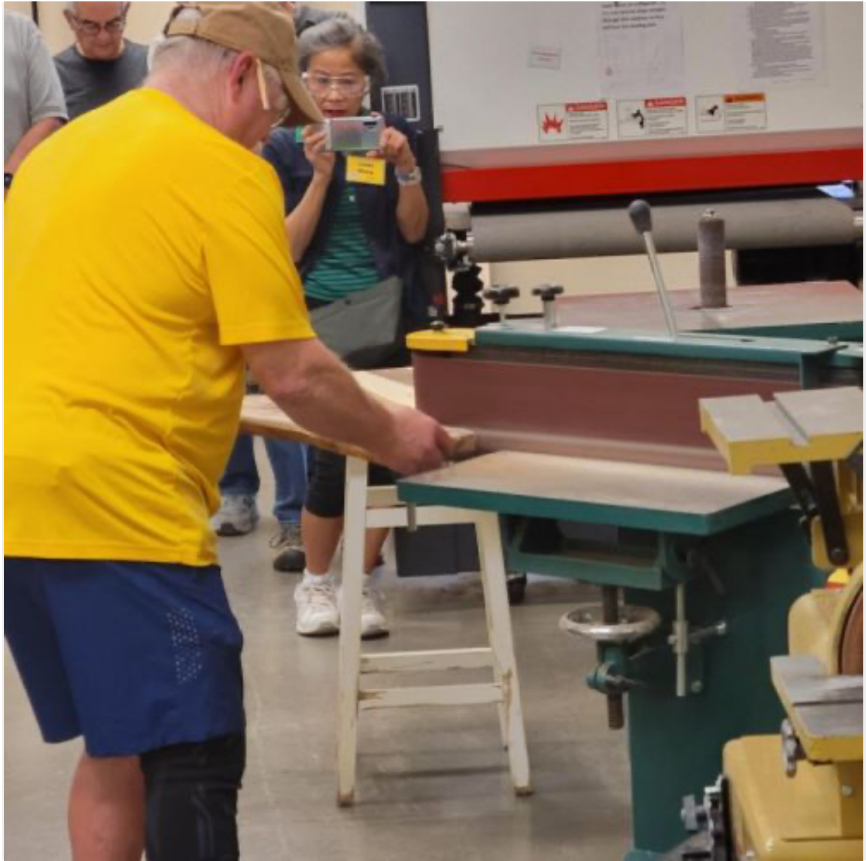
Horizontal sander is next to neaten up what the router didn't quite get. Also, a good time to remove any leftover bark.
